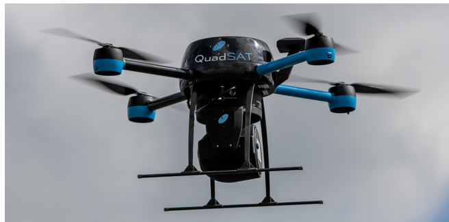
Fig. 1: QuadSAT’s compact UAS-APE. The compact gimbaled remote source antenna can be seen situated under the drone.
